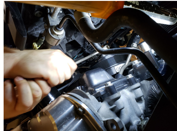
Reduced engine bay space seen in this Nissan GTR engine bay leads to higher underhood temperature.
