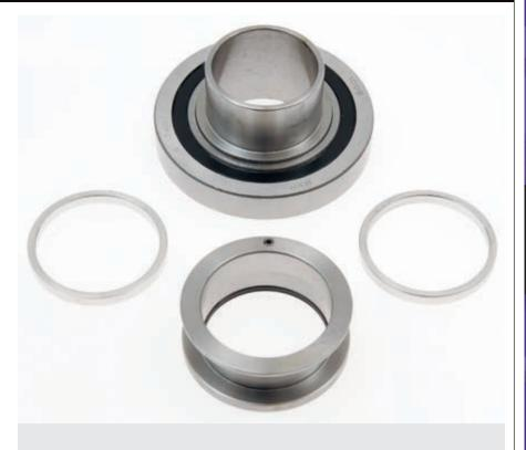
**3** McLeod makes a neat throwout bearing (P/N 16505) that solves many clutch linkage geometry issues. Years ago, you could purchase bearings in three different lengths, but that's not so easy today. You *can* get this cool adjustable bearing with removable sleeves that varies the length to either 1.325 inch, 1.525 inch, or 1.725 inch, which allows easy transformation to fit any clutch combo.
