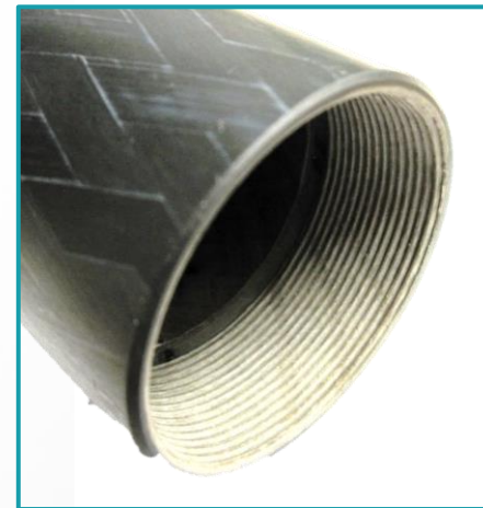
strut load introduction with co-consolidated thread (e.g. GF-PEKK)
