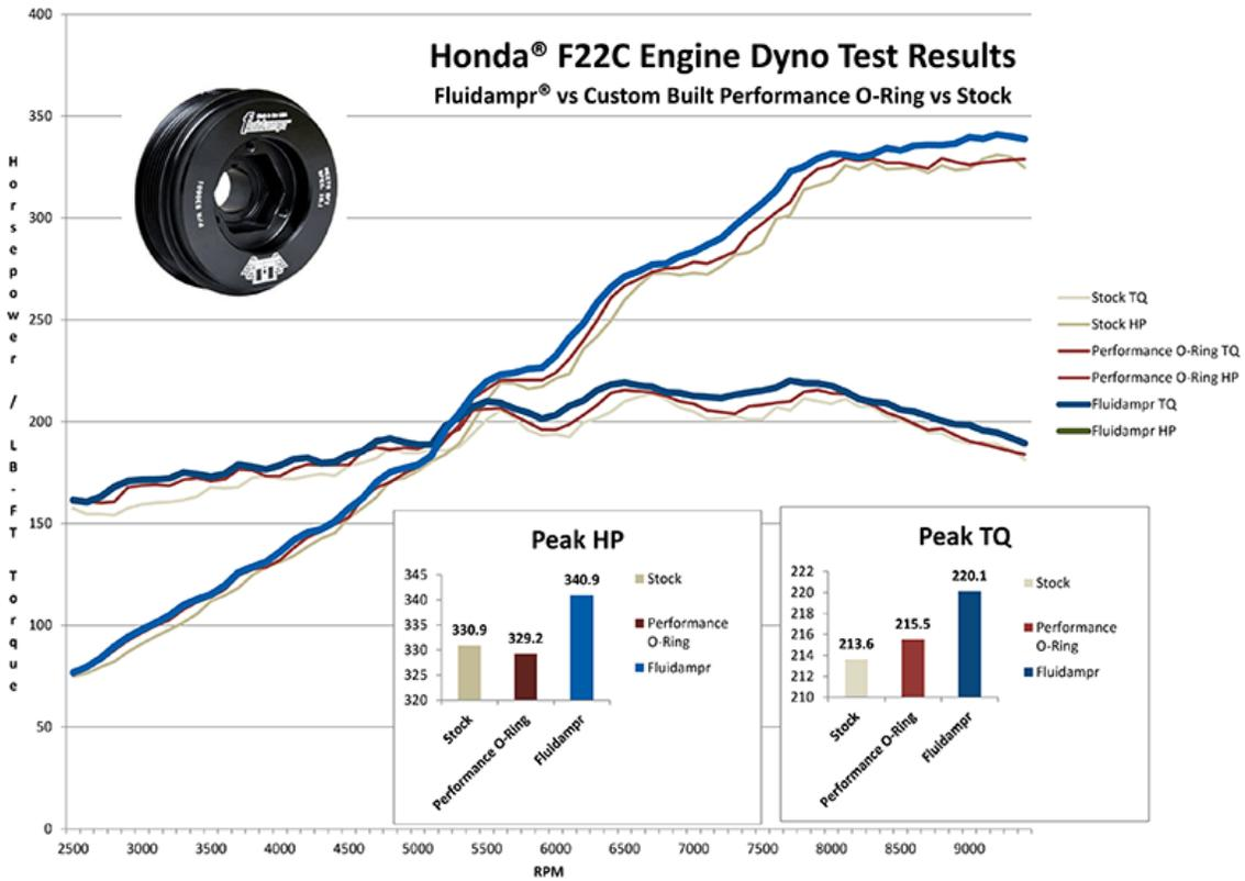
Controlled engine lab testing using a mildly tuned F22C engine on a Superflow water brake engine dynamometer at a rate of 1,000rpm per 2 seconds. Only the dampers were changed. Your results may vary.
