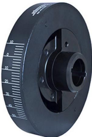
Fluidampr for 454-502ci external balance Chevy Big Block. The removable hub contains the counterweight mass. By changing only the hub this damper can then be used on an internal balance conversion.
