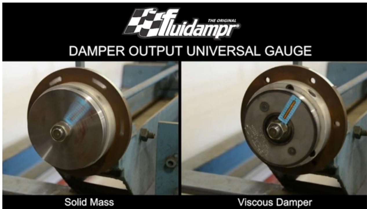
Side-by-side video of a five pound solid mass vs a five pound viscous damper on a validation test rig. When the torsion bar releases it throws each in motion to about 45°. The viscous damper (Right) stops moving in about 15 seconds, while the solid mass keeps moving well over 30 seconds later. [youtu.be/tNLersfbodE](https://youtu.be/tNLersfbodE)
