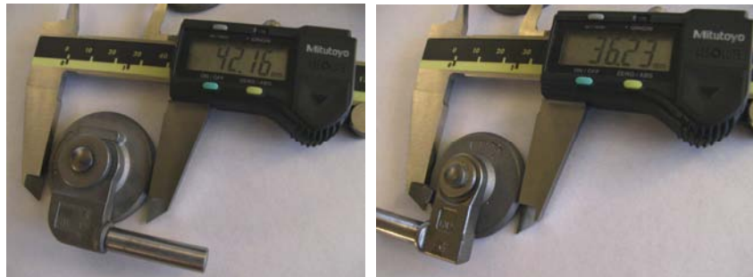
Figure 17: Wastegate Valves - 36mm and 42mm
