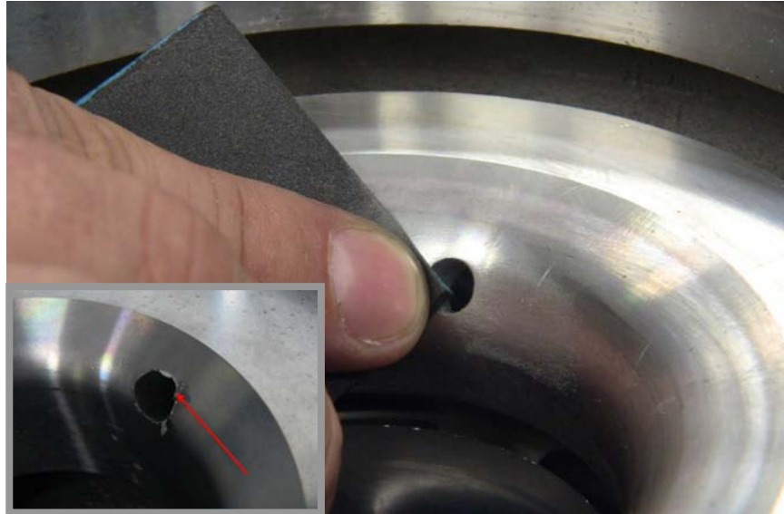
Figure 67: De-burring the Edge of Hole with Sandpaper
