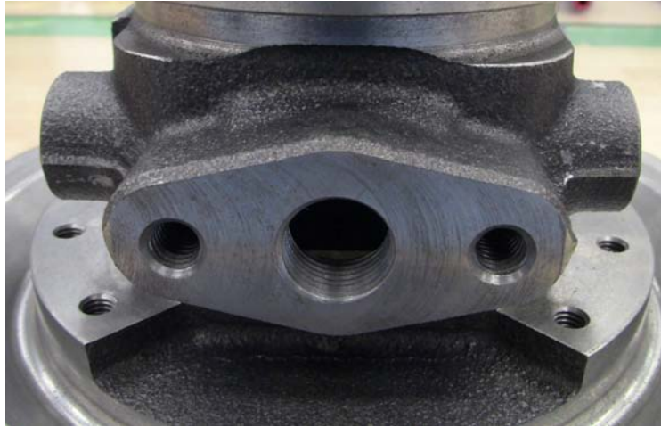
Figure 32: Oil Drain Pad Machined for Gasket and 3/8 NPT Fitting
