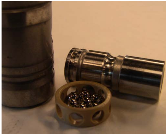
Figure 27: Competitor's Plastic Cage and Steel Balls
