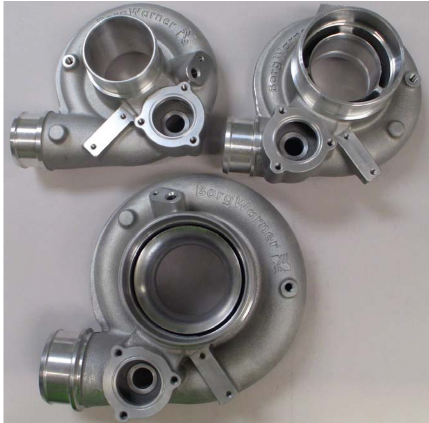
Figure 79: Compressor Covers and Their Inlets and Outlets
