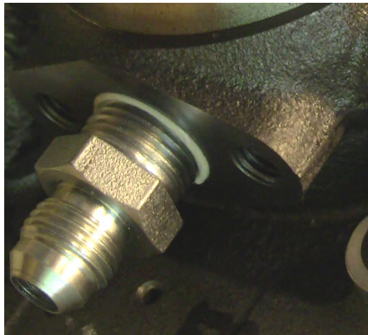
Figure 33: Oil Drain Fitting Installed (-8AN)
