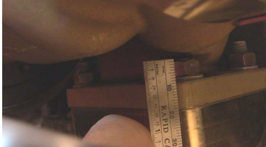
Figure 86: This Stud Position When Used With the "A" (0.65a/r) Turbine Housing Should Protrude No More Than 18mm From the Manifold Surface. The Nut Needs To Be Tightened On the Way Down.
