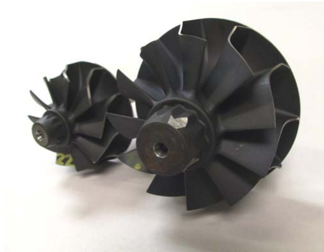
Figure 36: Gamma-Ti Turbine Wheels (55mm and 74mm Examples)
