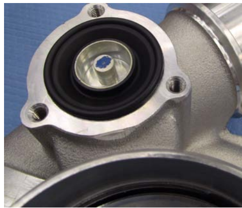
Figure 52: All EFR Compressor Covers Come Equipped With A Compressor Recirculation Valve, Which Can Optionally Be Disabled.
