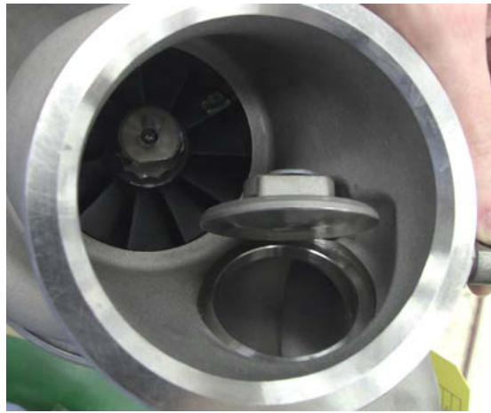
Figure 16: Large Internal Wastegate
