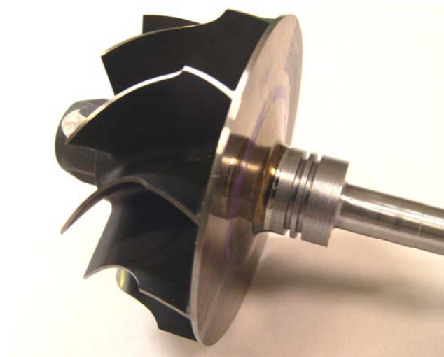
Figure 38: Gamma-Ti Shaft and Wheel Assembly (Superback + Fullback)
