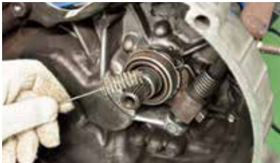
④ Apply the Grease to Top Shaft
