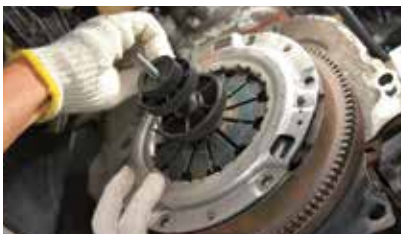
⑦ Installing to Fly Wheel
