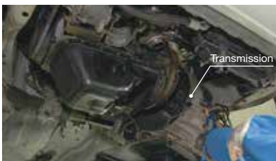
⑩ Reinstalling the Transmission
