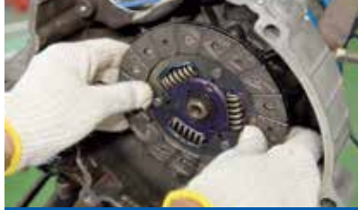
② Check for the Movement of Clutch
