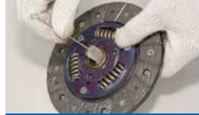
③ Apply the Grease to Spline Hub Teeth
