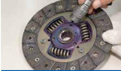
① Check for Clutch Disc Appearance
