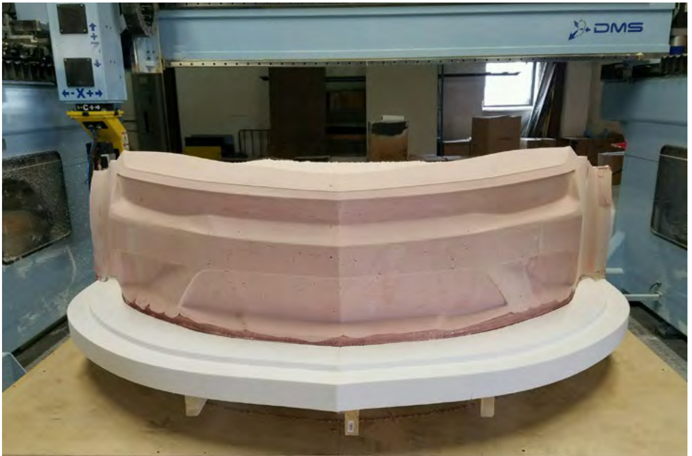
2017 ACP Camaro being cut on the 5 axis router
