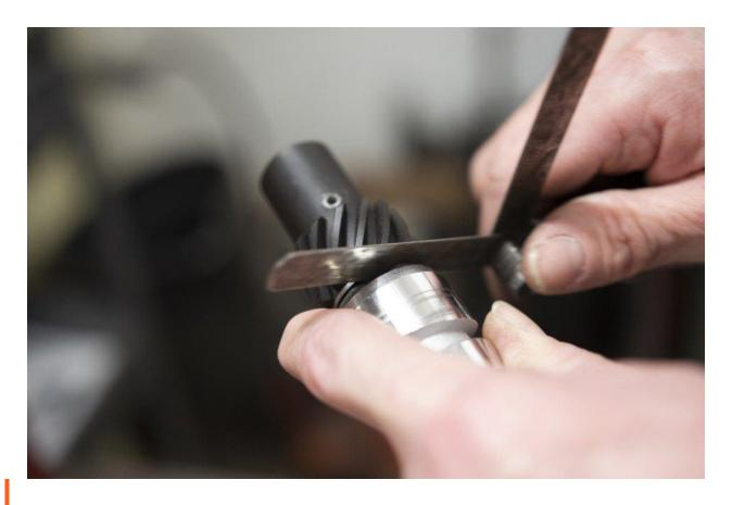
The gear's end-play is checked with a feeler gauge.
