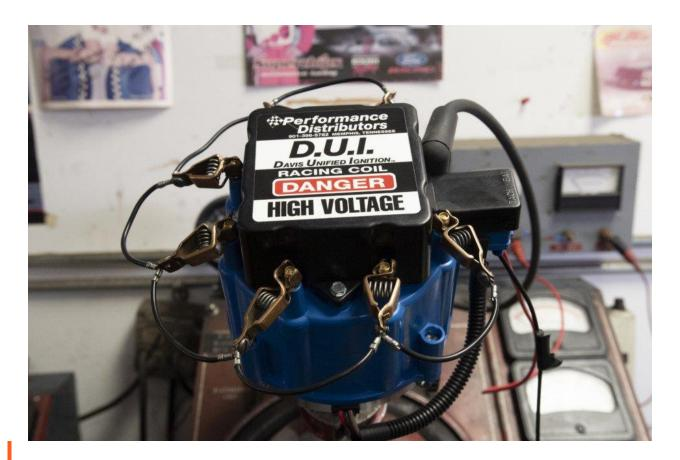
Test fired on the Sun distributor machine to ensure the unit meets specifications.
