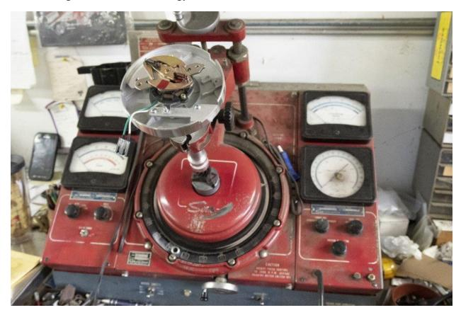
Every hand-built distributor is calibrated on a Sun distributor machine and test fired before shipping.
