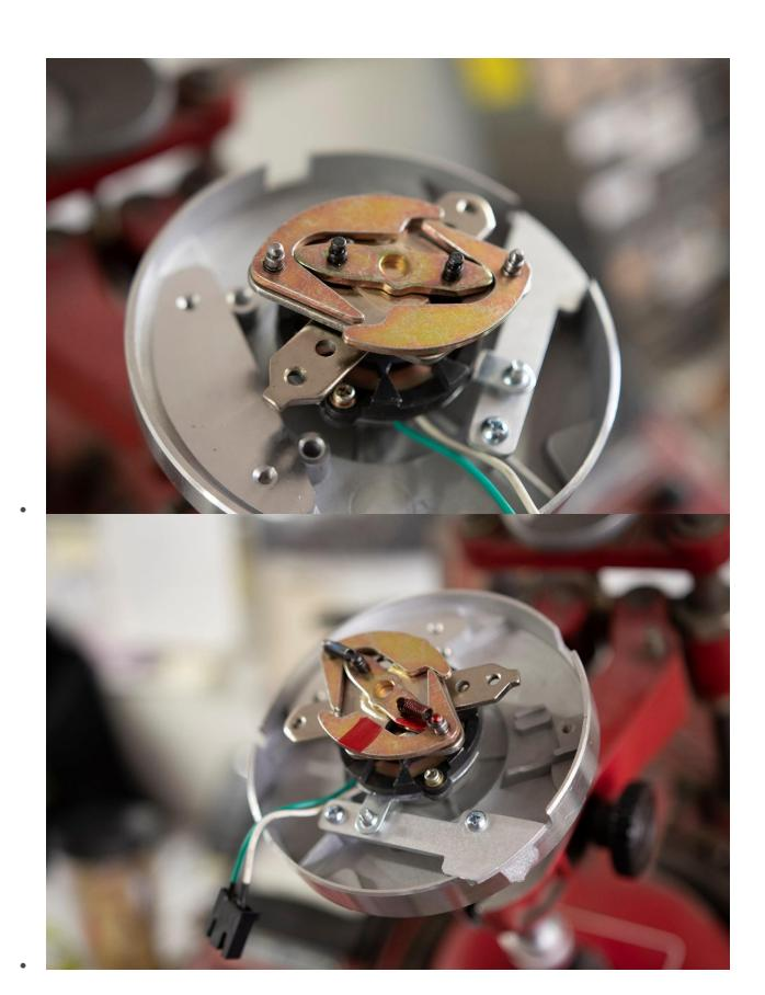
After the weights are installed, one side of the weights, springs, and ramps are color-coded red to help with future re-assembly. This ensures the ignition timing remains the same as it was when shipped.
