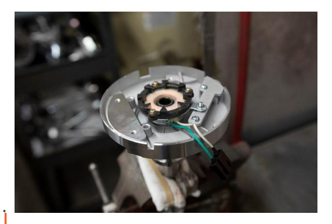
The housing gets fitted with ramps, blockout plates, and the timing ring prior to the inner shaft assembly.
