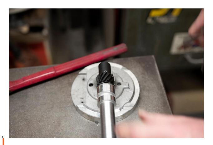
The drive gear is added to the bottom of the shaft and held in place with a roll pin.
