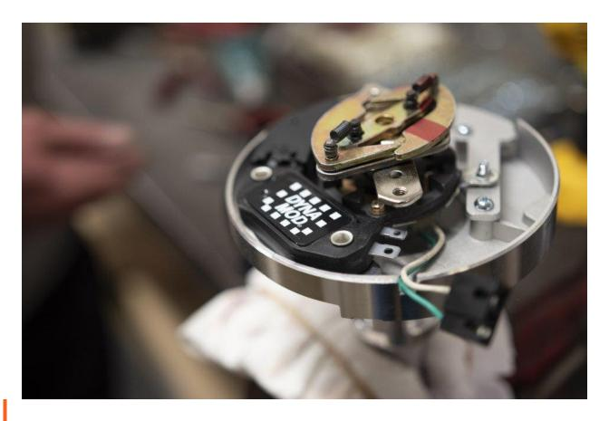
Completely assembled and waiting for the rotor and cap.
