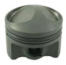
The pistons are machined from forgings with narrower and shorter skirts to reduce weight and friction. They are then dual coated, with Phosphate and MAHLE's proprietary GRAFAL® skirt coating. The phosphate is a dry film lubricant designed to help protect the pin bores from galling and ring grooves from microwelding. The GRAFAL® anti-friction skirt coating is designed to reduce drag, wear and noise.
