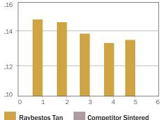
This graph depicts the tan material's coefficient of friction through each test level. Sintered data could not be obtained due to such early failure.
