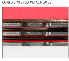
The red background light coming through the sintered plates indicates that the plates have severely coned resulting in failure.
