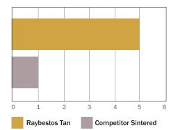
The sintered metal material coned and failed after just one test level while the Raybestos conventional tan material continued to perform.
