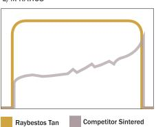
Tan material produces a smooth shift with an E/M Ratio close to 1 while the sintered material produces a harsh shift with a high endpoint.
