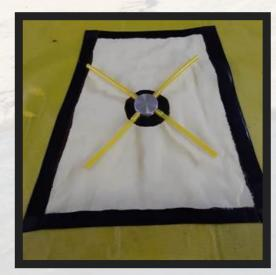
These pick-up hoses allow the elimination of the lift pumps and, consequently, of their hoses/fittings and power supply.
