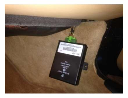
V. To install the DSC module onto the retaining bracket simply line up the upper tab and the bottom will snap into the locking tab.
