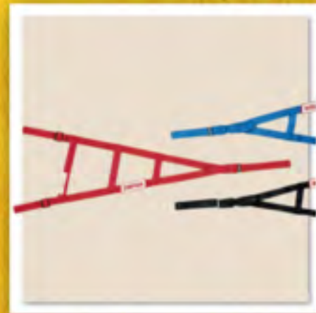
Head surrounds and/or side nets are critical in side impacts.
