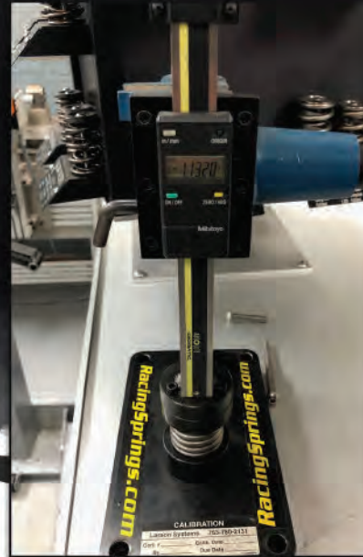
Solid Height Measurement
