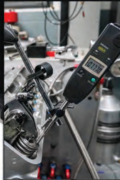
Actual Valve lift measurement (valve lashed)
