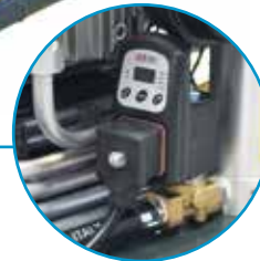
Automatic condensate drain with timer
