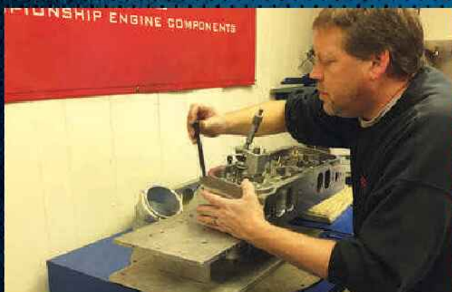
Traditional flow benches are still a useful tool in cylinder head development, but cannot provide any data regarding the fuel handling capabilities of a port or chamber design.
