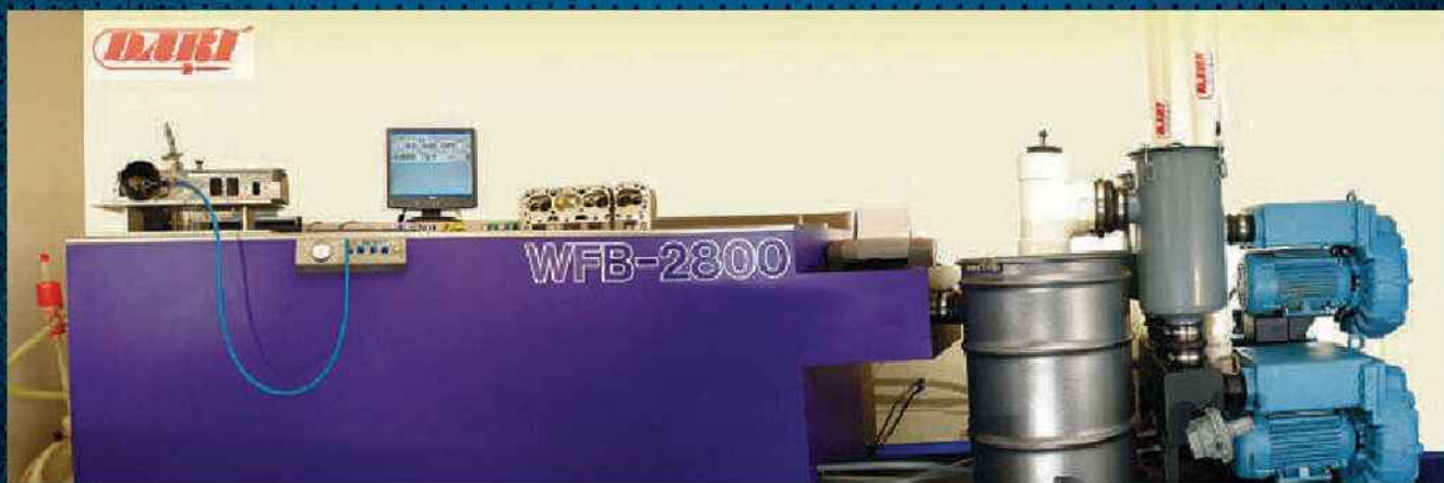
Dart's proprietary wet flow bench can flow 800cfm - with fuel in the mixture, and operates at 55 inches of depression rather than the 28 inches which is commonly used for testing dry flow. This more closely replicates the conditions present in an actual racing engine.
