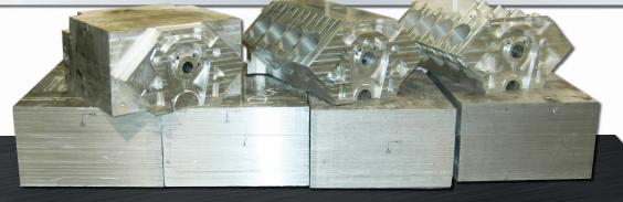
Precision machined from a solid Billet of Aerospace Aluminum, Dart Billet blocks offer virtually unlimited choices in bore centerline, deck height, bore diameter, lifter and cam options.
