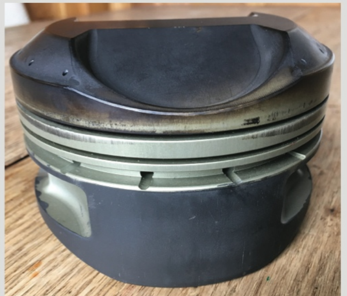
Fig. 3b: 3000hp, blown alcohol, hemi Pro Mod, 40 passes. Courtesy of Darrell Makins, Under Pressure Performance.
