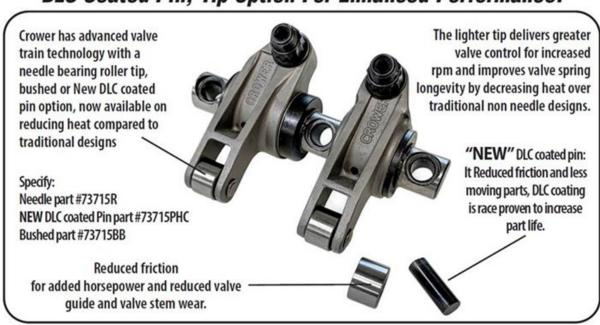
The needle bearing design minimizes friction, resulting in increased horsepower and less wear on the valve guide and stem. The DLC-coated pin further reduces friction with fewer moving parts. This race-proven technology has been shown to extend component life.
