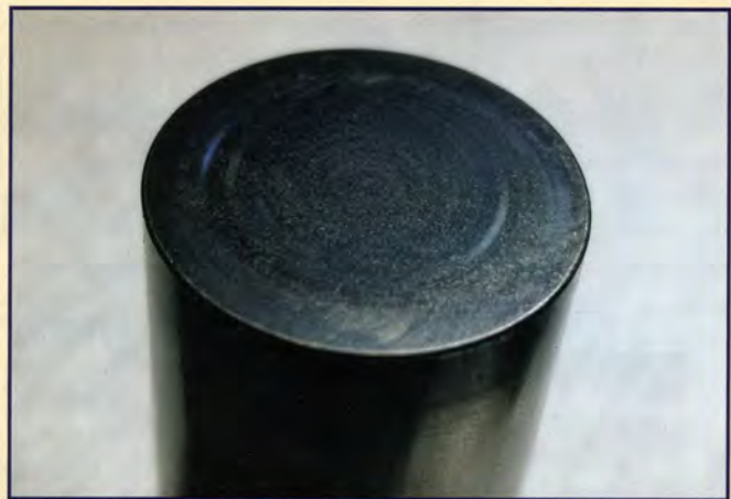
This is an picture of a hydraulic flat-tappet lifter with normal wear. The original convex surface can be worn either flat or concave as long as it is worn to a specific cam lobe. There can be many miles left on this combination of lifter and lobe if the right lubrication is used.
