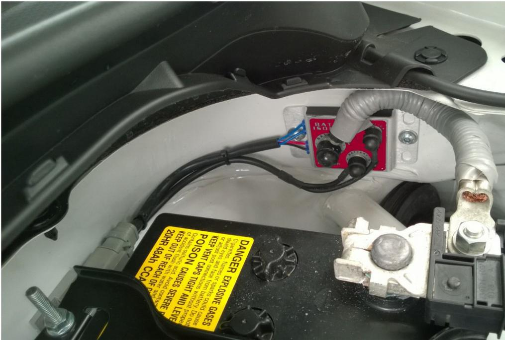
The Isolator should be mounted directly to the vehicle's metal chassis close to the vehicle's battery but away from any high temperature sources.
