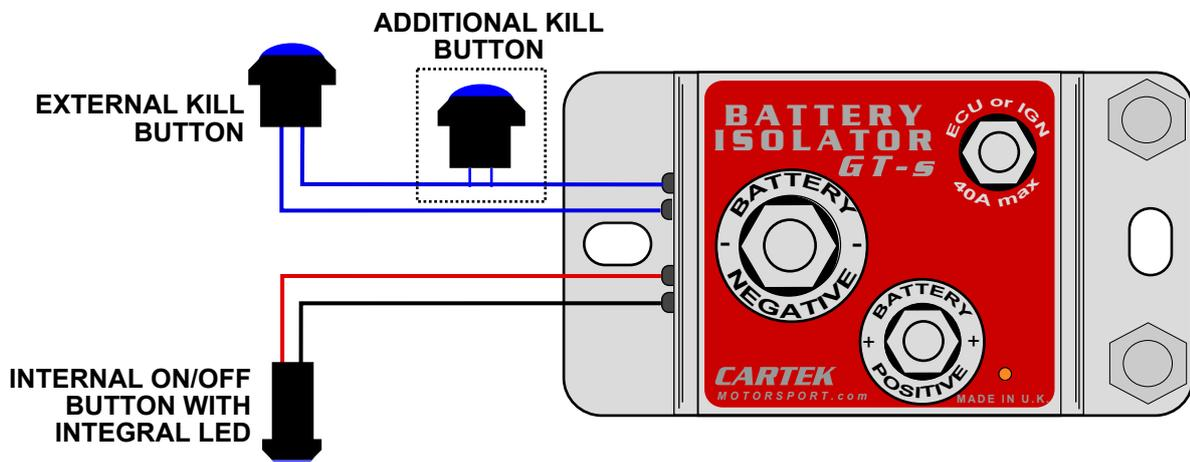
**CARTEK Battery Isolators** allow for an external 'kill' button to be mounted on both sides of a race car for instant access and maximum safety.
