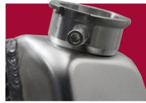
A billet filler neck is manufactured to SAE specification for performance and safety. Includes correct overflow tube on all muscle car applications. Interior weld for professionally finished look.
