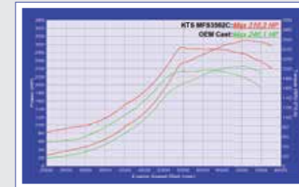
Only change of wheels and boost from 1.0 to 1.3 bar, no further modification
