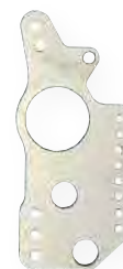
Housing bracket • integral wheelie bar mount • water jet cut • 3/16" thick • 1/2" holes • fits 3" axle tube P/N 40-135-2 (Mild Steel) 40-135CM-2 (Chrome Moly)
