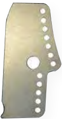
Frame bracket • water jet cut • 3/16" thick • 1/2" or 5/8" holes • for use with S&W frame rail 10-410-01 • notched for 1-5/8" crossmember P/N 40-135-1 (Mild Steel) 40-135CM-1 (Chrome Moly) 10-410-4L(5/8" holes)
