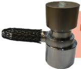
Resting the housing on the Press Insert tool, locate the bearing into the housing with the half of the staking tool.
