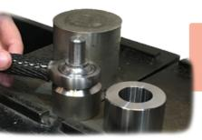
Remove the staking tool from Press Insert tool and check to ensure the bearing is centred in the housing.
