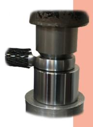
Ensure that the bearing is inserted fully into the housing.
