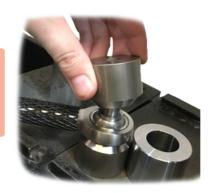
Apply the staking force with the press onto the staking tool, ensuring the staking tool is in proper and full contact with the staking grooves.
