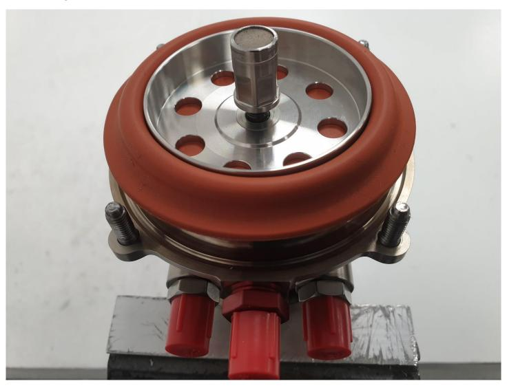
Torque the magnet-nut to 14Nm using a 'crow's foot' type socket.
