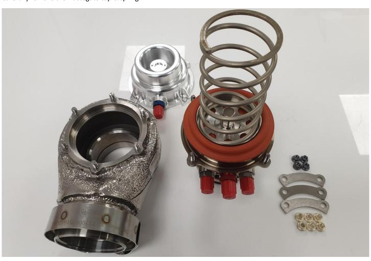
Clamp the wastegate valve head in a vice using aluminium jaws. Be sure not to clamp the heatshield.
