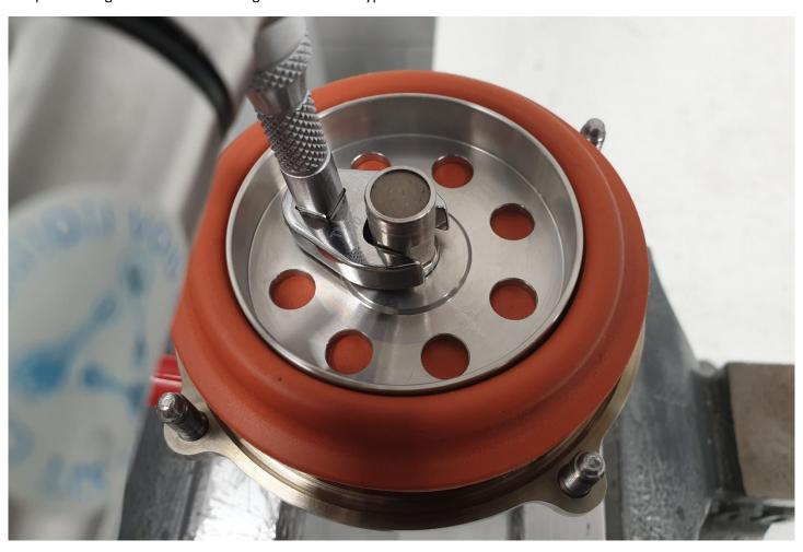
Remove from the vice & clean off any excess Loctite from the magnet-nut. Refit the spring & cap.
