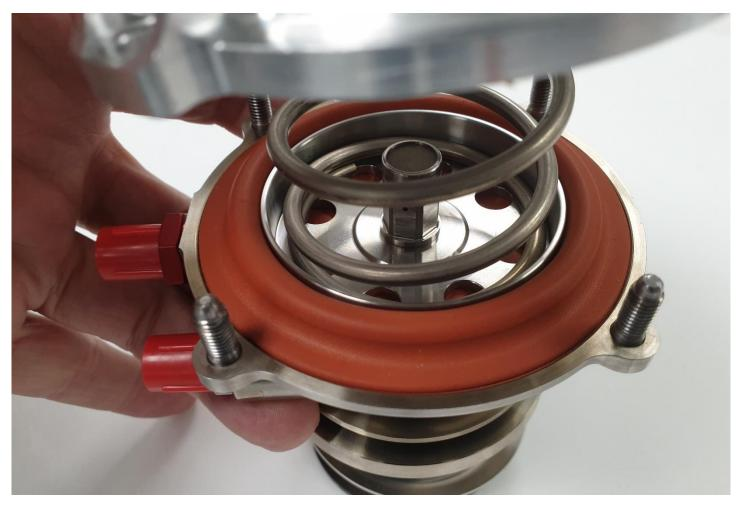
Torque the x4 M5 Knuts to 7Nm.
