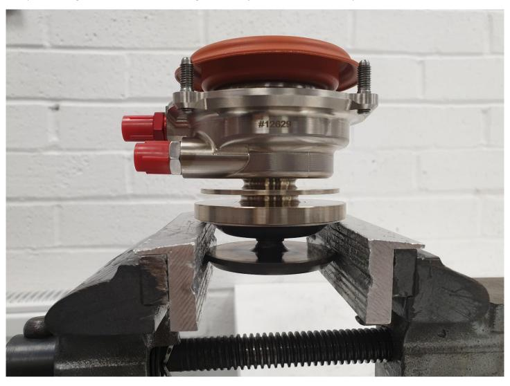
Remove the M6 washered Knut from the valve stem.
