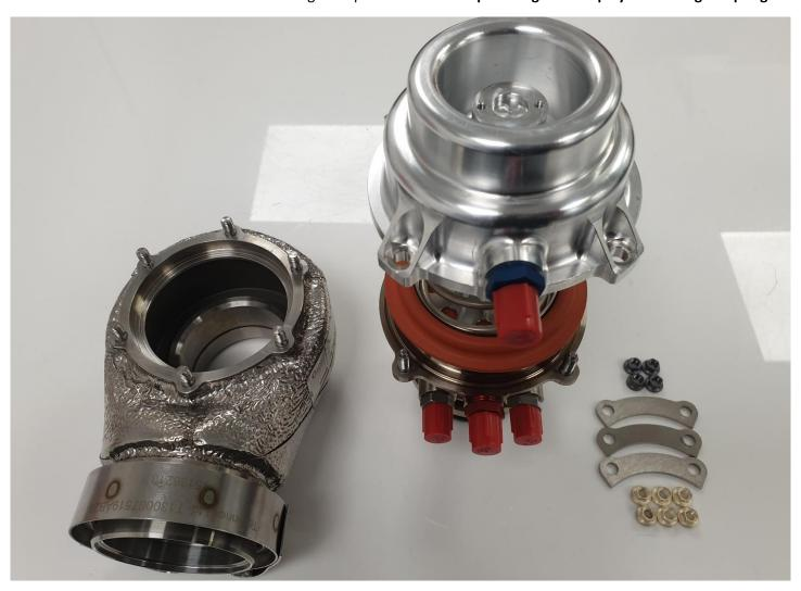
Carefully remove the wastegate cap & spring.
