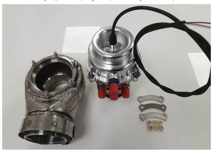
Refit the wastegate to the casting assembly using the 3 retaining plates & x6 HT Knuts.
