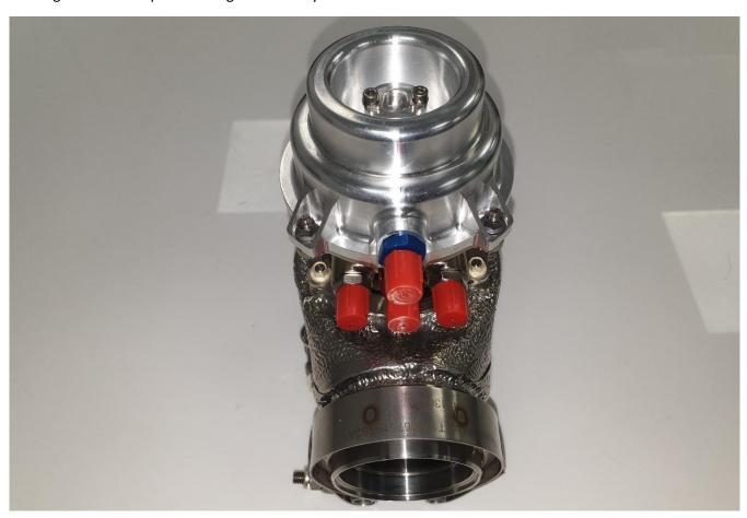
Remove the wastegate from the casting assembly.
