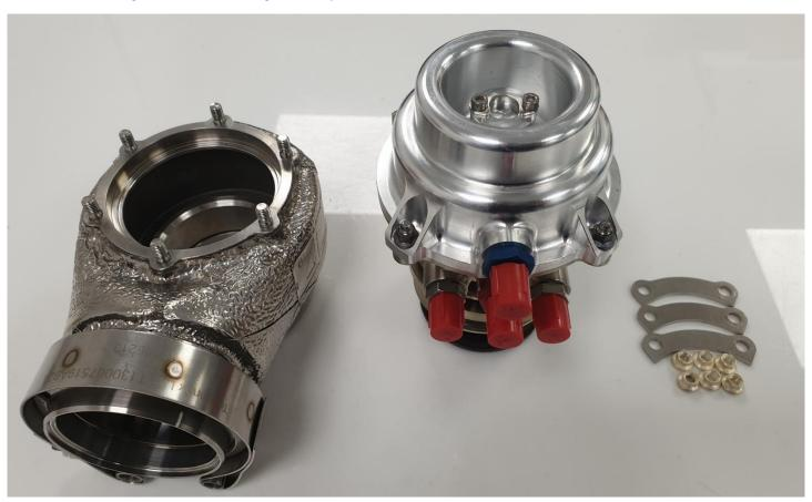
Remove the x4 M5 Knuts to release the wastegate cap. Caution – the cap is being forced up by the wastegate spring.
