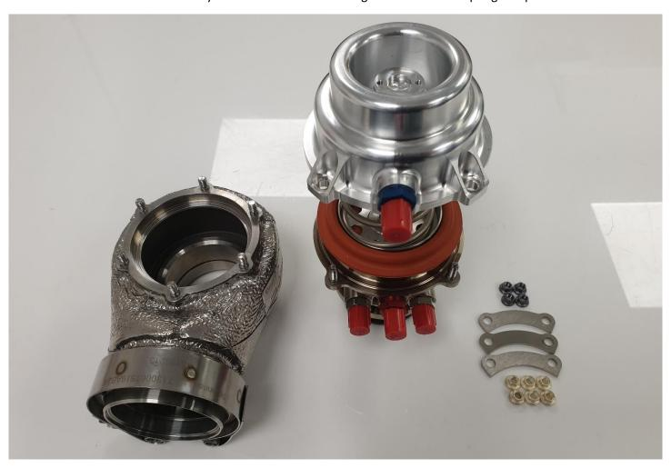
Lift the main body up & ensure that the diaphragm is seated correctly. Push down on the cap against the spring & refit the x4 M5 retaining Knuts.
