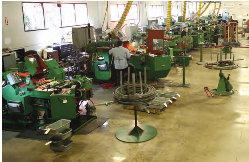
ARP's bank of cold-headers can handle material up to 5/8" diameter and form bolts in a multi-phase operation.
