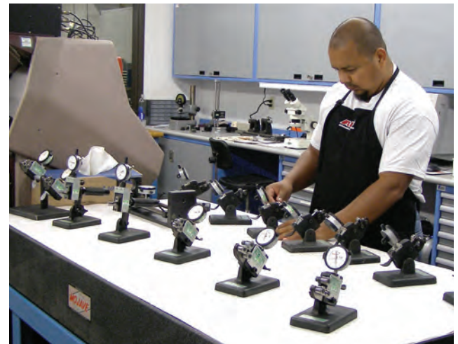
A series of special checking devices are employed to monitor the quality of threads. For every thread size, there is a checking device.
