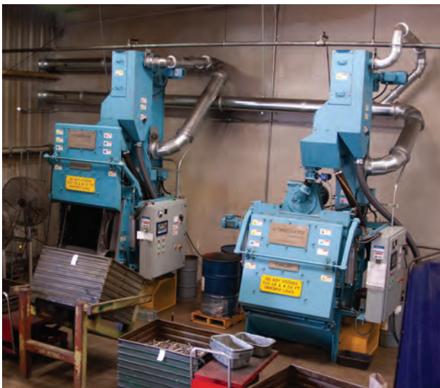
Fasteners are shot-peened to improve fatigue life.
