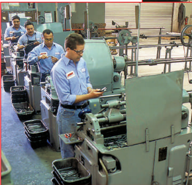
Lengths of bar stock are automatically fed into special machines and cut to the appropriate length.
