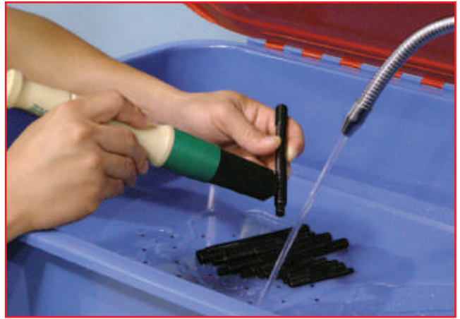
2. Clean and inspect all hardware prior to installation, looking for shipping damages and defects.
