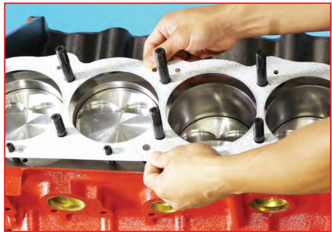
4. Install gasket and head, then lubricate the stud threads, the washers and nuts with ARP Ultra-Torque fastener assembly lubricant prior to their installation.
