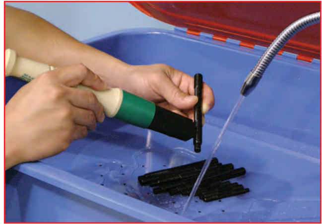
2. All hardware should be cleaned and inspected for possible shipping damage prior to installation.
