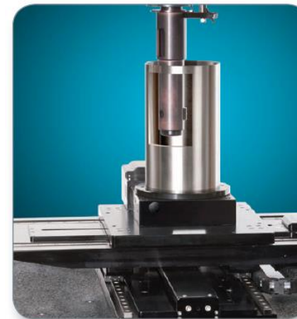
Bore-Scope objective collecting data 150 mm inside large metal engine cylinder liner.
