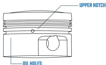
The oil ring side rails are supplied with one or two tabs. One is installed with the tab facing the side of the groove designed to lock the rail using one of the grooves in the piston. The other tab (if applicable) is designed to lock the middle expander. Use at the top or the bottom is the same.
