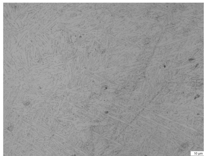
Figure 5a. As-built microstructure of L-PBF Ti6Al4V, showing almost 100% acicular \alpha' martensite with some nano-scale retained \beta (adopted from [1])
