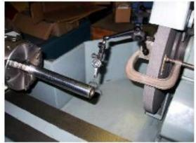
Use the infeed wheel to move the indicator back far enough to clear the test bar. Then go in the same sequence to the right to check each measuring point. Use the infeed wheel to advance the indicator over the top of each measuring point to find the high point.
