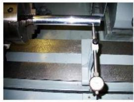
Zero the test bar in the tailstock the same way. The problem with this type of check is that the slightest bump of the test bar can move it so be careful!
