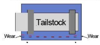
do not apply enough pressure to hold the head or tailstock solid against the table which will aggravate the problem. Cleaning and lubricating the hold down bolts is important to help prevent this from happening.
