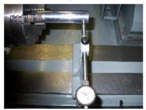
from center after clamping. If you cannot easily get bar stock Joe Baker Equipment Sales has test bar stock for sale.
