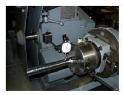
When your machine is far away from the ideal numbers it can be very difficult to get a round journal when grinding. Since normal wear will move the tailstock toward the wheelhead and point the test bar down quite a bit, top shoe steady rest pressure will push the crank further away from the bearing centerline. Heavy bottom shoe pressure might help bring it up toward the centerline of the bearings.
