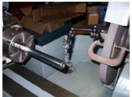
Now rotate the grinding wheel so the indicator is just clear of the ground surface. Move the indicator to the next measuring point and slowly rotate the grinding wheel until the indicator reaches the high point. Record that number, + or - of the zero reading you had set on the indicator at the first measuring point.
