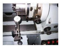
Even if you have an air floated head and tailstock and have always cleaned them carefully before moving you can have this type of wear. The cause is the force created when you offset the chucks and counterweights for grinding rod throws. Even though you do not see any movement when the machine is running it is constantly trying to rock the head and tailstock back and forth. It is also common to have the hold down bolts get rusty so they
