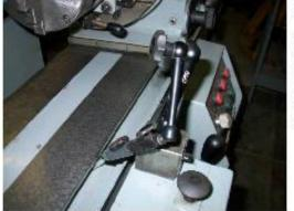
Next we want to check the table for wear. You can attach an indicator to the grinding wheel, grinding wheel spindle housing or the gearbox on the front of the machine.
