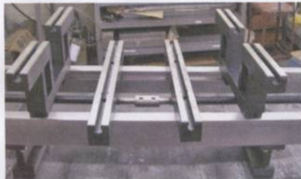
For inline blocks use the proper set of parallels for the cutting height.
