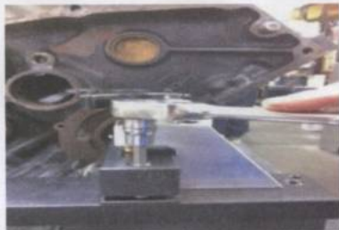
Level block long ways with the leveling adjustment screw on the block roll over bar.
