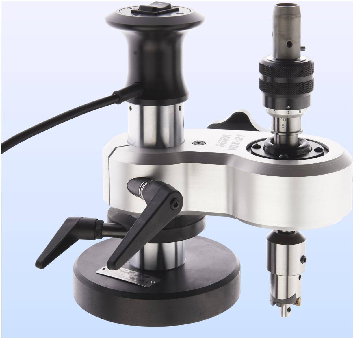
The portable VGX-21 valve seat refacing unit has been developed for the specialised petrol and diesel cylinderhead workshop. The highly accurate valve seat processing is achieved by a spherical spindle guide bearing as well as a unique hydraulic ball clamping system. A almost pressure free centering and braceless fixing of the MIRA rotary head is made possible in order to achieve precise and concentric valve seats ! **Order Number: VGX-21**
