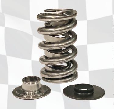
Designed for maximum endurance in sustained high RPM dirt late model applications employing super lightweight valve components: (7mm diameter intake and 5/16" diameter exhaust valves) along with titanium valve locks, lightweight "tool steel" retainers and large dia/heavy wall pushrods. Coupled with the above components, the natural frequency separation of the Centrifugally Dampened<sup>™</sup> #1410ML yields superior valve control over any current valve spring designs.
