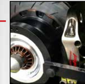
Frame Designed for Additional Brake Caliper Clearance
