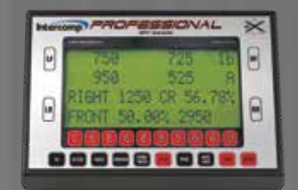
Weights Displayed on RFX™ Indicator & in RaceWeigh™ Software Simultaneously
