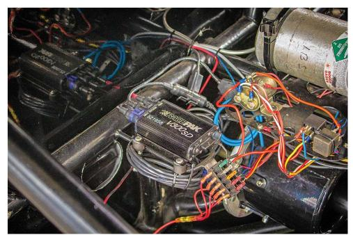
Interference on the sensor itself can affect data logging, so moving to remote mount sensor blocks may help avoid harmonics. "Subjecting your sensor to [vibration] will cause false readings and lead to a premature failure. Routing sensor wires away from high-powered ignition components is a must," our source from Holley told us.
