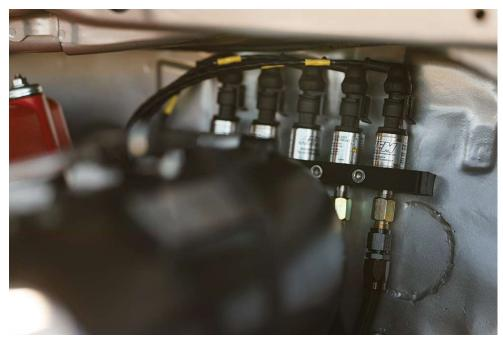
Material selection determines how precise of a reading sensors can achieve, as noted by a source from AEM Performance Electronics. "Upgrading from our brass type to stainless sensors are recommended for accuracy when you are using them for tuning and data analysis. We like to say it's the equivalent of the difference between using a ruler and using a caliper to measure something. Both will measure, but one will measure with a higher degree of accuracy," he said.
