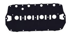
Foamet product line features an aluminium core and both sides coated with expanded nitrile rubber, then coated with silicone release coating to ensure excellent result in characteristics upon disassembly. Foamet gaskets are used mainly for breast plates or in exhaust gasket system as per engine.
