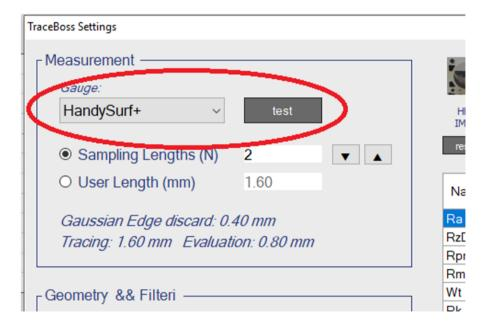
Launch TraceBoss (with the Handysurf+ connected). Click on the Settings gear and select "HandySurf+". Click the "Test" button to verify communications.
