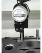
Electronic Level For precision leveling of valve guides (Canted Guide Fixture shown).
