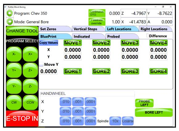
There are three (3) different modes you can operate the machine in on these screens, Blueprint, Indicated and Probing.
