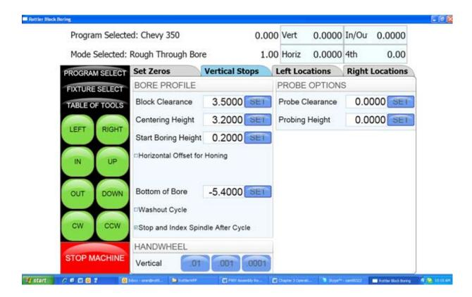
The Vertical stops have now been set. You are finished with the Vertical Stops screen, select Left and/or Right Locations.
