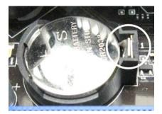
Remove the battery and place new battery in the battery holder.
