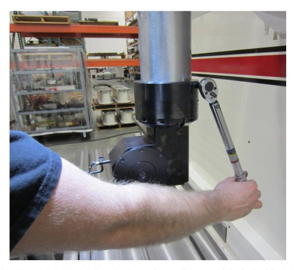
Tighten the two hub clamping bolts located at the rear of the unit. Tighten to 30 ft. lbs. (41 N m ) Recheck Alignment and re-adjust if necessary.
