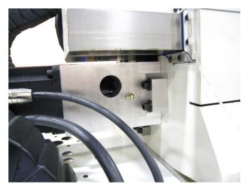
Z-Axis Grease Fitting is located at bottom of Ballscrew in spindle housing. Open cover to gain access.
