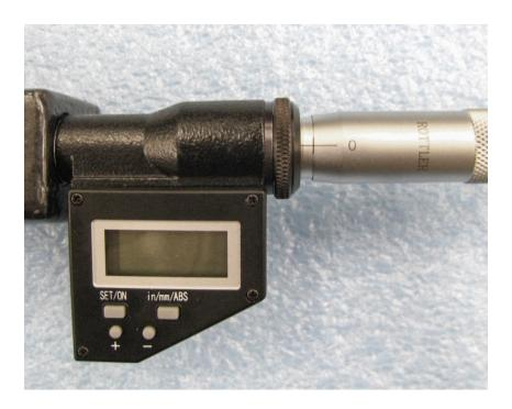
Determine which cutter head bore range the micrometer is going to be used on. (example; 2.9-6.0) We want to initially set the micrometer to the minimum bore diameter of this cutterhead.
