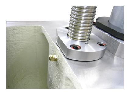
Oiler Reservoir is located inside the oiler door on the right side of the spindle column.
