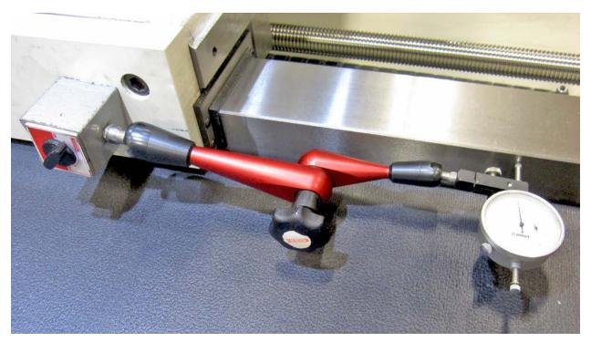
Now using the handwheel in .010" per click mode, move the column back and forth, about two turns on the handwheel in each direction at a rapid rate.
