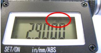
Press and hold the set/on button and the + or – button at the same time. "Set" will flash in the display. This places the micrometer in edit mode. (CAUTION: use a pencil tip or something similar to gently push the small round buttons - they are quite small and a bit delicate.)
