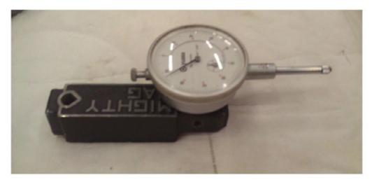
If the axis is overshooting or coming to position slowly you will be able to see it with a dial indicator. With Digital indicator you will only see the end position. The Magnascale indicator should be used to dial or tram in. The automatic moves of the machine can "Shock" the sensitive plunger of the Magnascale.
