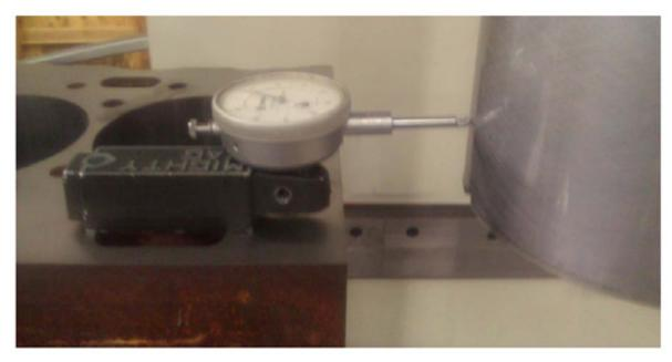
Bring the spindle of the machine in position to put a slight load on the Plunger, about .020". Set "Vertical, Horizontal, In/Out" zero.
