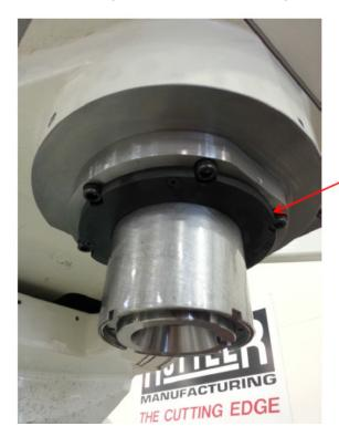
Retainer - O-Ring and felt are underneath
