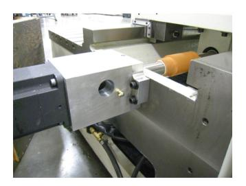
Y-Axis Grease Fitting is located on the back of the spindle above the electrical enclosure.
