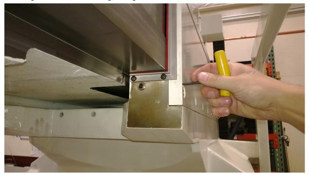
2. Put the machine in "Mill Cycle" mode, with the wedge turned off. Attach an indicator as shown in the following photo, and set to zero position.
