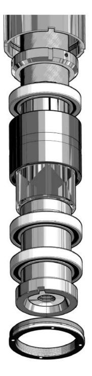
Install 3<sup>rd</sup> bearing with the closed side down.
