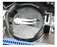
Using your finger tip push down on the battery until the retention clip is in its lock position.
