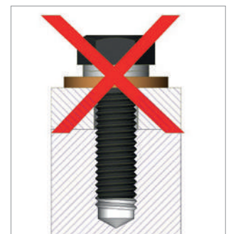
No locking function when combined with flat and freely rotating washers
