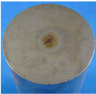
Lifter Cam Face after the EDM oil hole burned showing the Recast area.
