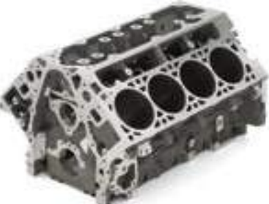
LT1/LT4/LT5 Aluminum 6.2L Bare Block (top, front)
