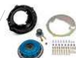
19331080 Transmission Installation Kit Includes Super Magnum steel bell page 30
