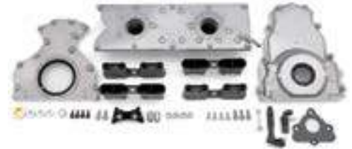
Gen III Bare Block Completion Components
