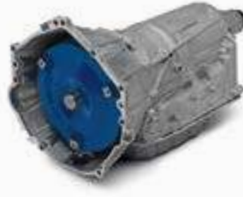
19366637 or 19417102 SuperMatic™ 6L80-E Six-Speed Automatic page 26
