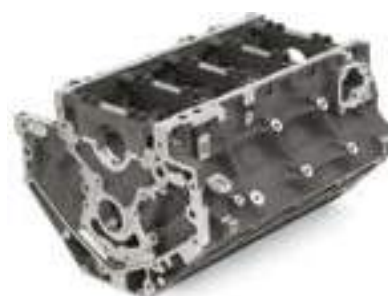
LT1/LT4/LT5 Aluminum 6.2L Bare Block (bottom, rear)
