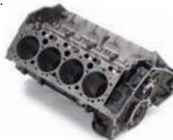
Production-Based Block (top, rear)
