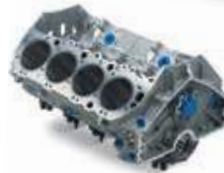
ZL1 Aluminum Big-Block (top, rear)
