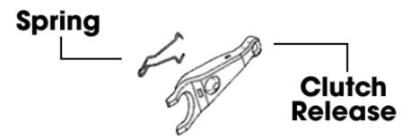
Failure To Do So Will Cause The Fork To Rub Against The Pressure Plate
