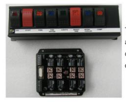
This system is an example of using an 8 switch panel and 8 circuit controller, it can be used in a turbo or supercharged application.
