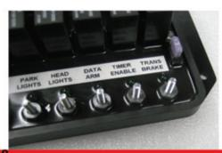
12 relay controller configures for turbo cars with data arming and timer enable circuit. When the transbrake is applied to the input on the relay controller it will activate the transbrake relay circuit and disarm the timer enable circuit, you release the transbrake and the timer enable circuit becomes active again. This feature is commonly used with EFI systems and data logging.
