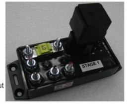
full throttle switch will activate the positive trigger allowing you the versatility to activate any output with any signal. We use slow blow fuse rather than ATO style fuses for any of our high current products eliminating the possibility of a high current spike that will blow a guick reacting fuse upon solenoid activation in hot high temperature conditions.
