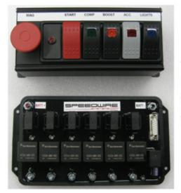
Typical layout of 6 switch panel with Mag shut off option. Each circuit is fused and incorporated LED status on fuses and outputs.
