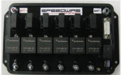
This controller has 6 (50 amp rated) circuits and has self diagnosing LEDs for fuse and output staus, if a fuse blows the LED will turn from yellow to red. When the relay is activated the output LED will turn green.
