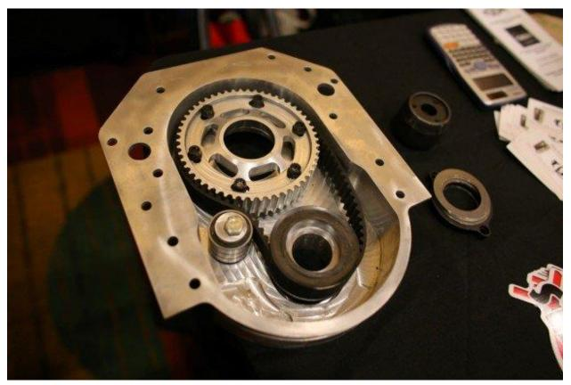
The company has also developed a billet belt-drive system for use on the block that allows the user to pull the camshaft out as a cartridge, keeping the Torrington bearings intact and simplifying the cam-swap process.
