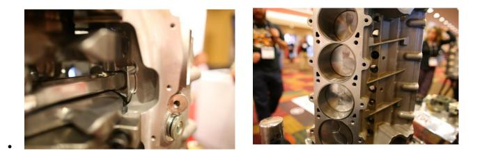
(Left) Even at bottom dead center, there's still plenty of cylinder covering up the pistons. (Right) Titus has outfitted the block with an 18-head-bolt configuration and can provide the block unmachined, or tuned up and ready to go.
