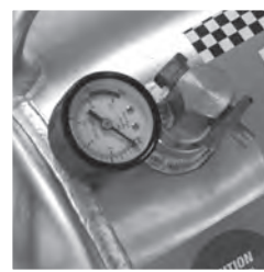
Built-in pressure gauge shows tank pressure
