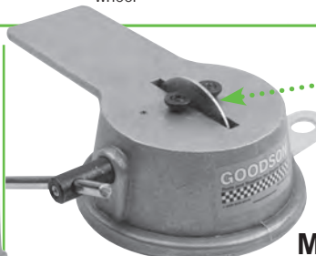
4 Table pivots past grinding wheel
