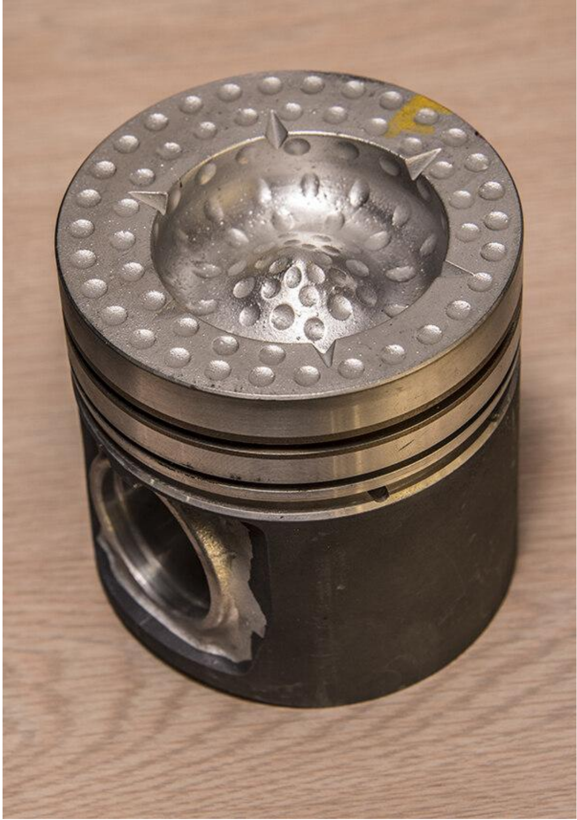
This closeup of the SOA piston head shows the intricate pattern and shapes of indentations needed to improve the flame front.
